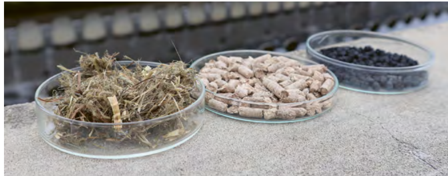
The path to biogenic activated carbon: on the left, grass-like landscaping material; in the centre, pellets produced from it, which were processed into biogenic activated carbon (right) via pyrolysis and activation.
